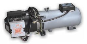
The **DBW 2010** hydronic heater offered by Webasto will heat up to a 48 foot sailboat or a 47 foot powerboat. The **DBW** 2010 utilizes 3/4" water hose to deliver heated coolant to fan heaters throughout the boat. The DBW 2010 uses a 1-1/2" rigid exhaust system, and a 1/4" supply and return fuel system. The **DBW 2010** is available in 12 or 24 volts.
