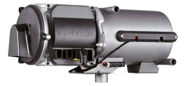
The **Thermo Top Pro 150** hydronic heater offered by Webasto will heat up to a 48 foot sailboat or a 47 foot powerboat. The **TTP150** utilizes 3/4" water hose to deliver heated coolant to fan heaters throughout the boat via a 110 volt pump. The **TTP150** uses a 1-1/2" rigid exhaust system, and a 1/4" supply and return fuel system. The **TTP150** is available in 12 or 24 volts.
